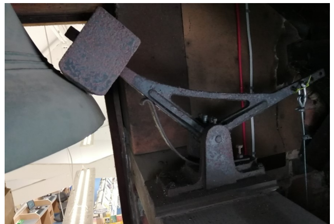
Church House Bell and triking mechanism linked to the clock
