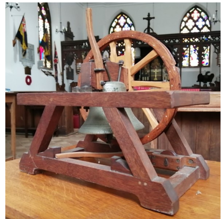
St Peter's model of a bell in the down position with the "stay" upright
