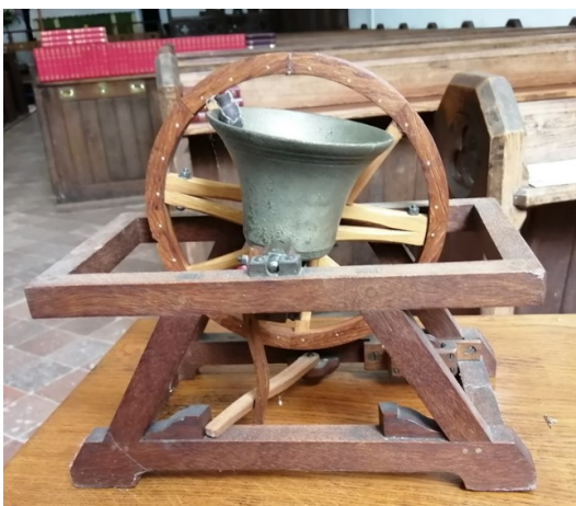
St Peter's model of a bell in the ringing position with the "stay" against the slider
